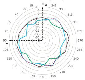
Elevation plane (side view, 0 degrees angle) - 5 GHz
